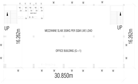
SHED 1 - OFFICE FIRST FLOOR PLAN
