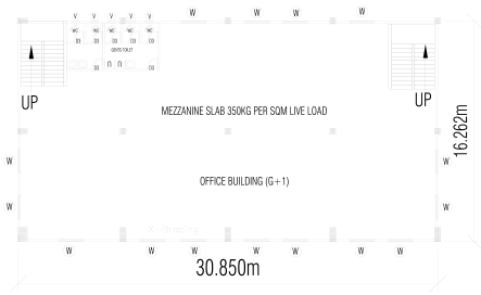
SHED 2 - OFFICE FIRST FLOOR PLAN
